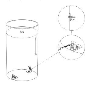
9. Apply a thick bead of adhesive silicone caulkling to the base of basin where it meets the floor.
